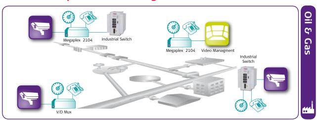
Fast and reliable communications are vital for maintaining secure and safe operations of gas or oil platforms, rigs or distribution pipelines. RAD offers a range of aggregation multiplexers and industrial Ethernet switches to handle the transport and concentration of real-time monitoring and control data, SCADA, telephony and video communications over fiber, copper or wireless links.
