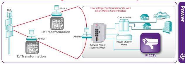
One result of the evolution to Smart Grids is the deployment of Smart Meters in residential areas. These meters enable bidirectional communications with the power control systems and billing applications.
